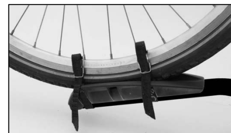
Figure 15: Tensioning straps for front wheel
